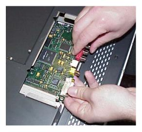
Gently push the board into the connector. The board is fully seated when the four screw holes (six for the SDI board) are aligned.
